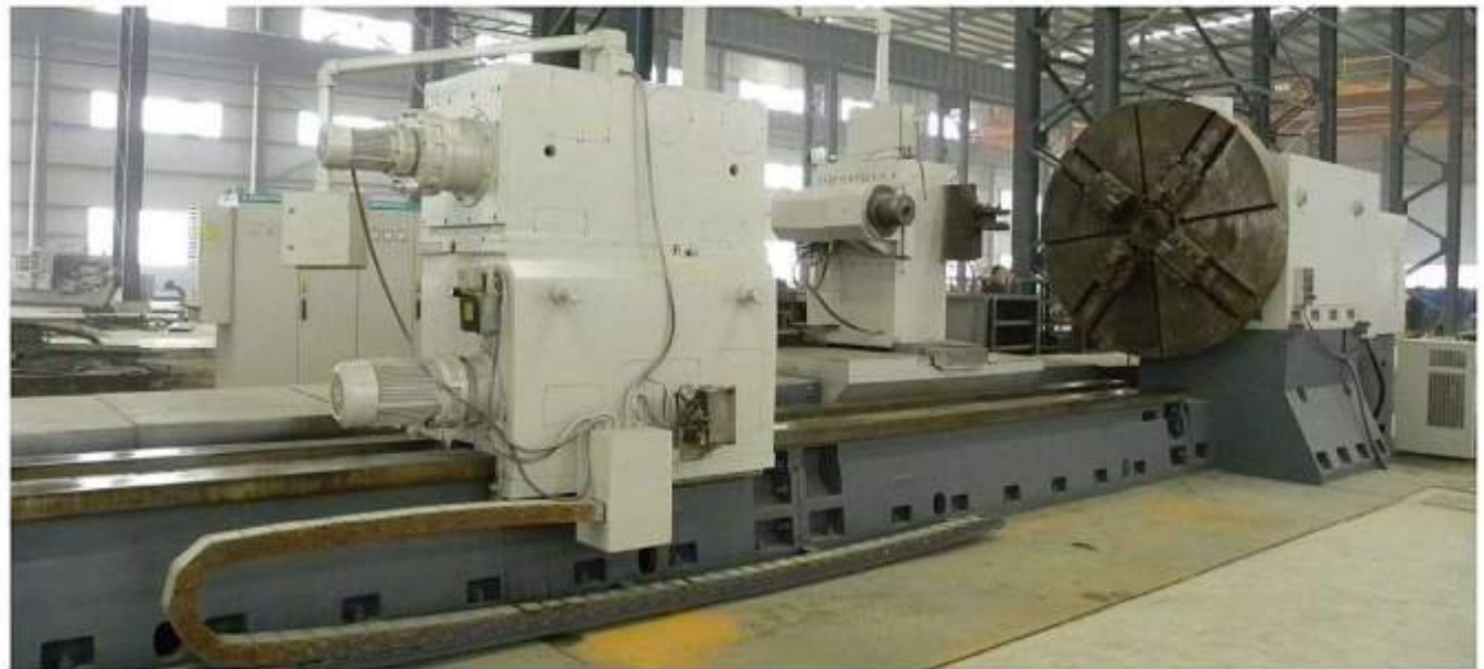
数控重型卧式车铣中心CH612206M CNC Heavy-duty Horizontal Milling Center CH612206M
