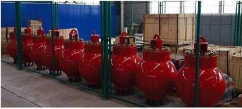
F系列泥浆泵锻件空气包总成 F-series forged Pulsation Dampener Assembly (45-75L)
